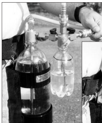
Spray bottle is being refilled through extended brass tube.
