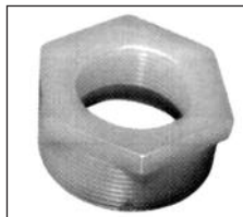
RB1418-NY: 1/4" npt(M) x 1/8"(F) reducer bushing. RB3814-NY: 3/8" npt(M) x 1/4"(F) reducer bushing.
