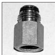
2KGF-O 5/8"-18(M) x 1/4" NPT(F) stainless adapter for Firestone spray side plug.
