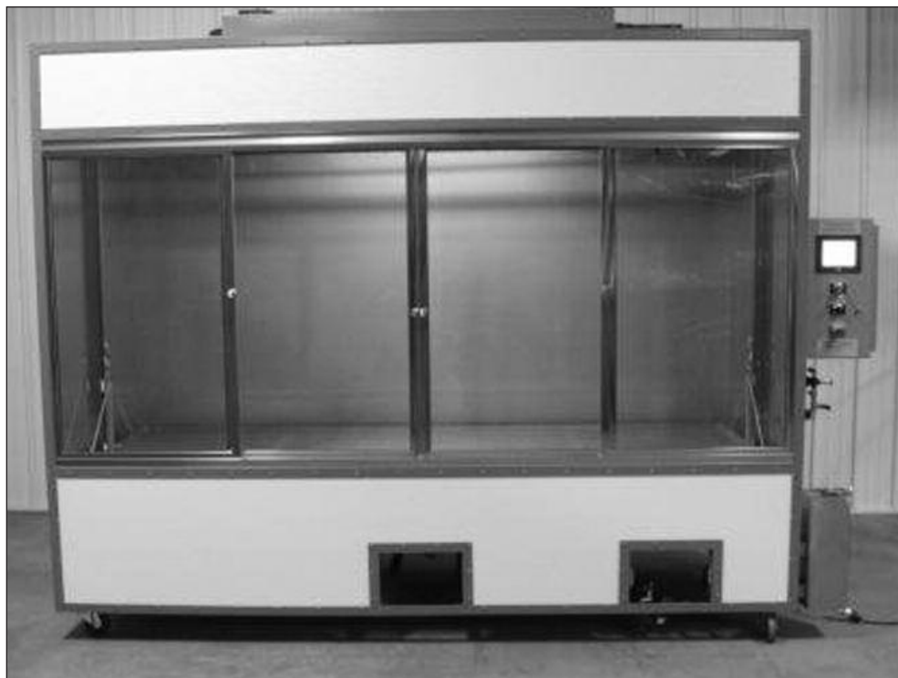
SB8: Shown with rainfall nozzle, solvent flush, electrically powered stainless steel shelf and standard touch screen controls
