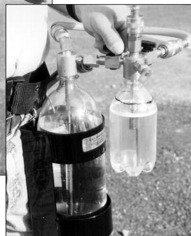
Spray bottle is being refilled through extended brass tube.
